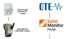
There is a clear graphic image on the Portal incl. values from electrometer for consumption and production.
